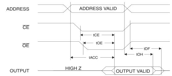
Notes: 1.  $\overline{CE}$  may be delayed up to  $t_{ACC}$  -  $t_{CE}$  after the address transition without impact on  $t_{ACC}$ .
