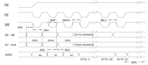
Notes: 1. A0 - A14 must conform to the addressing sequence for the first 3 bytes as shown above.
