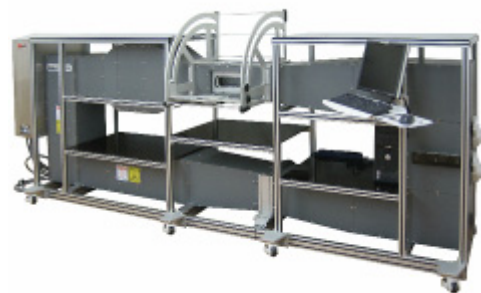
Fig. D: FDK Original Wind Tunnel
