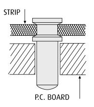
100 Contacts on a polyester strip, packed in a tube, ideal for multiple loading. Strip can be easily cut into any length and left in place, or removed after soldering.
