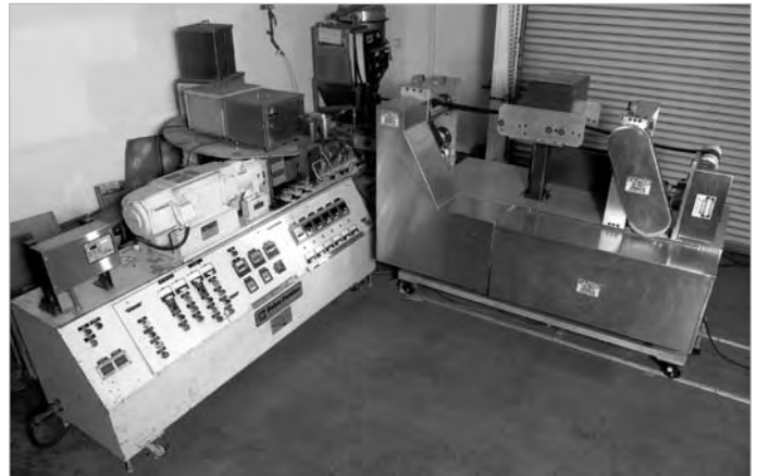
Thermoplastic extruder for microwave absorbing thermoplastic products.
