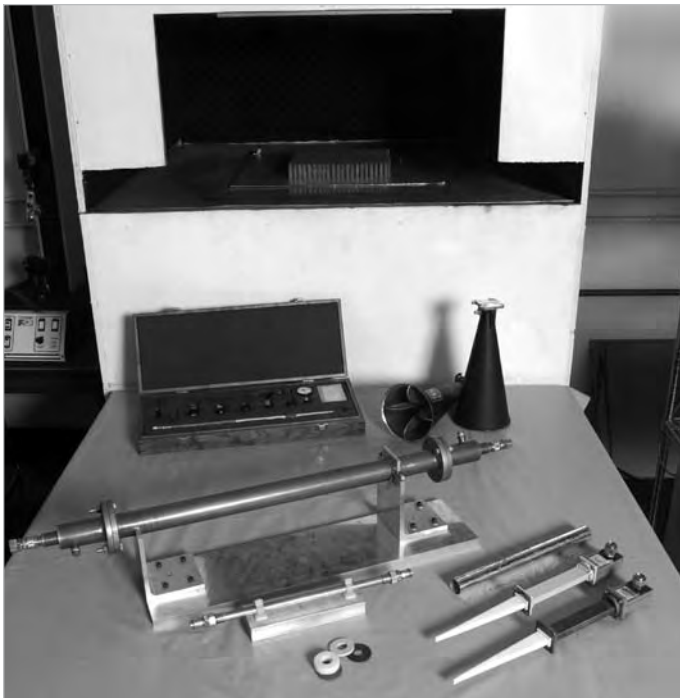
Transmission tunnel and microwave test equipment for material property measurement.
