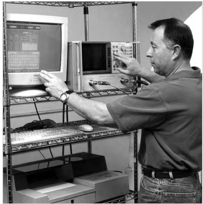
Computer controlled network analyzer provides amplitude and phase measurements on microwave absorbers.
