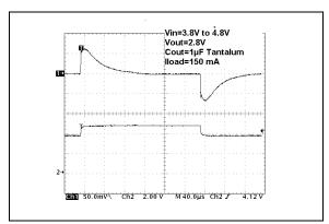
**FIGURE 2-14:** Line Transient Response 1  $\mu$ F Output Capacitor.
