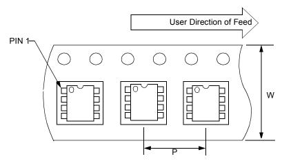
Standard Reel Component Orientation for TR Suffix Device
