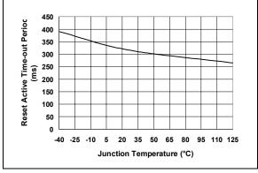
**FIGURE 2-4:** Reset Active Time-out Period vs. Temperature.
