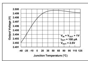
**FIGURE 2-3:** Normalized  $V_{OUT}$  vs. Temperature.
