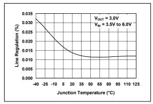
**FIGURE 2-1:** Line Regulation vs. Temperature.
