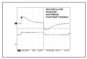
**FIGURE 2-16:** Line Transient Response 10 μF Output Capacitor.
