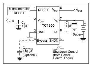
FIGURE 3-1: Typical Application Circuit.
