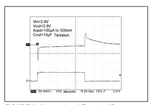
**FIGURE 2-15:** Load Transient Response 10 μF Output Capacitor.
