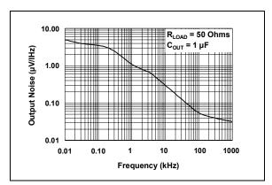
FIGURE 2-5: Output Noise vs. Frequency.
