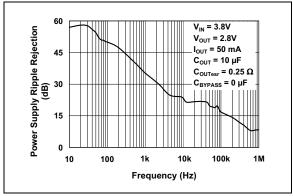
**FIGURE 2-7:** Power Supply Rejection Ratio vs. Frequency.
