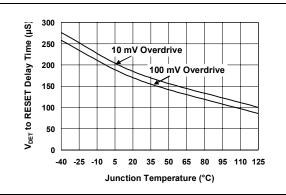
**FIGURE 2-12:**  $V_{DET}$  to Reset Delay vs. Temperature.
