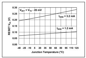
**FIGURE 2-17:** RESET Output Voltage Low vs. Junction Temperature.
