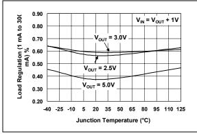
**FIGURE 2-9:** Load Regulation vs. Temperature.
