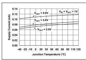
FIGURE 2-2: Supply Current vs. Temperature.
