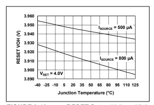
**FIGURE 2-18:** RESET Output Voltage High vs. Junction Temperature.
