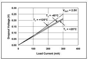
FIGURE 2-6: Dropout Voltage vs. Load Current (2.5V).
