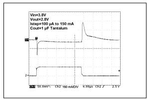
**FIGURE 2-13:** Load Transient Response 1  $\mu$ F Output Capacitor.
