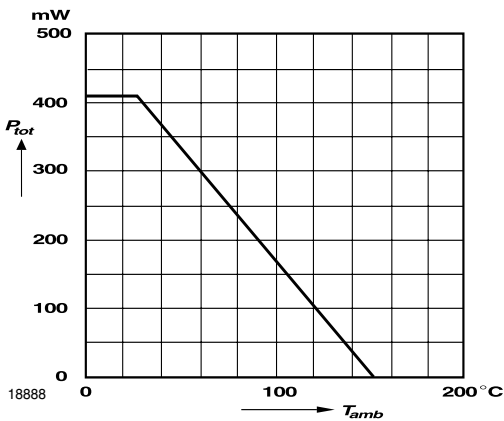
Figure 2. Admissible Power Dissipation vs. Ambient Temperature
